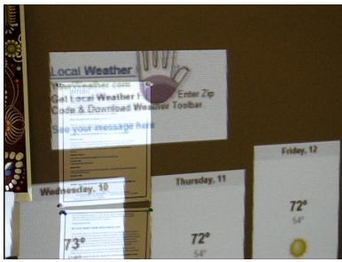
Figure 7: SURROUNDWEB maps natural gestures to mouse events. Here, the user uses a standard “push” gesture to tell SURROUNDWEB to inject a click event into the web application.
